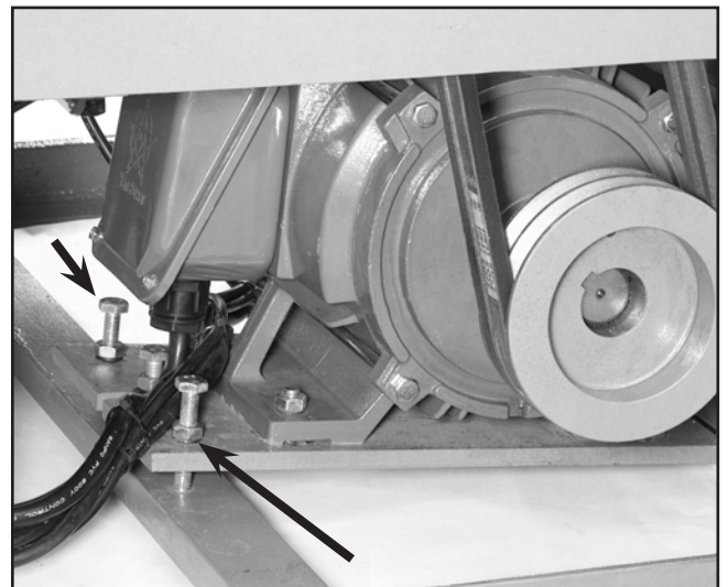
Figure 23. Motor mount adjustment bolts.
